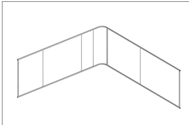
**Step 5:** Unzip print and lay image face up. Slide print onto frame like a pillow case. Grip the fabric tightly and stretch around bottom pole to pinch zipper into place. Zip the graphic together for taut finish.
