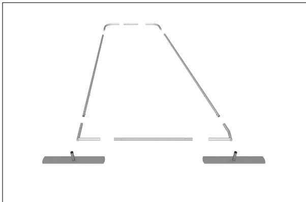
**Step 2:** Connect all corner sections to curved and straight sections of the frame by matching shape symbols on pipes.
