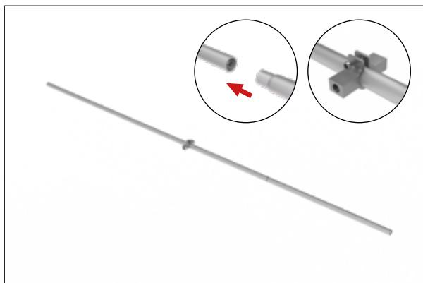
**Step 5:** Join the 2 vertical side frames to top and bottom horizontal frames while placing the center support pole into position.
